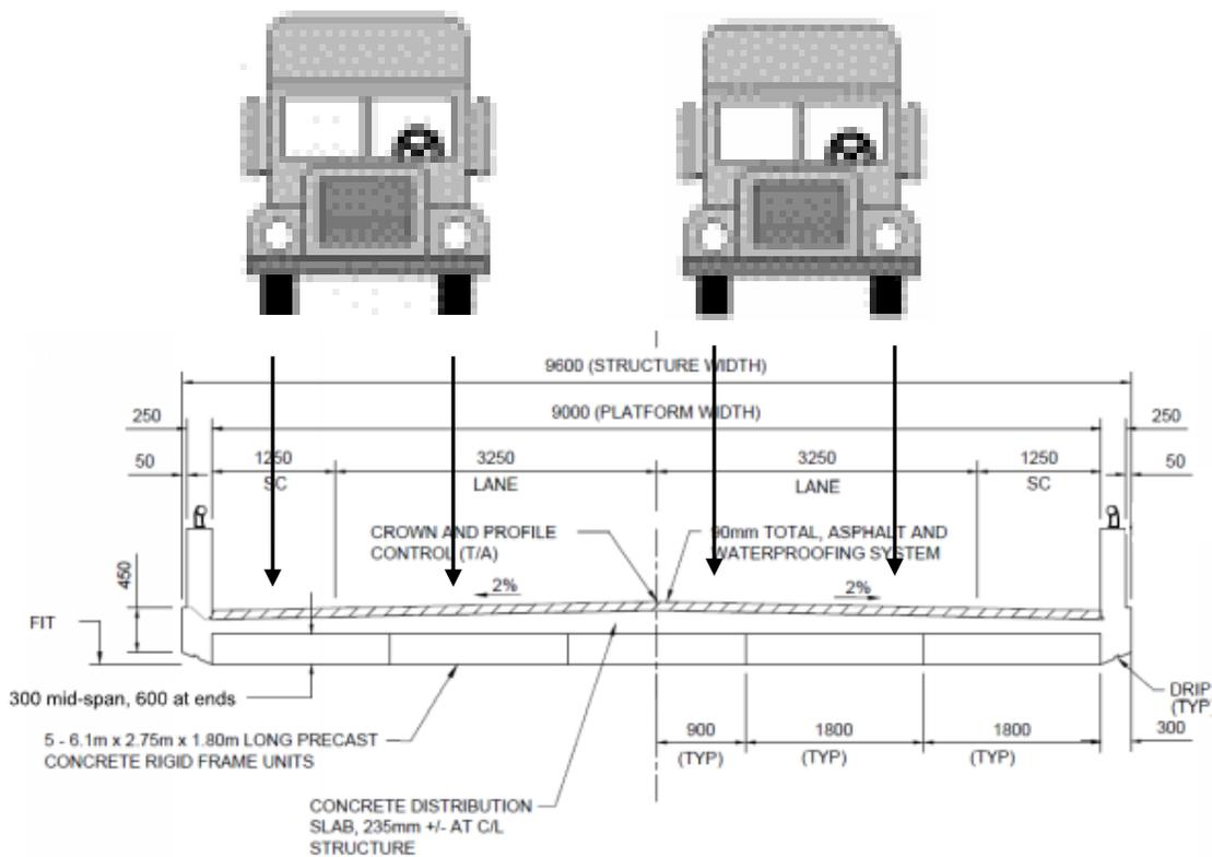
The live load after applying the multi-lane factor can be applied as a concentric load on a footing that is  $(0.25 + 0.6 + 1.8 + 2.1 + 0.6 + 1.8 + 0.6 + 0.25) = 8.0\text{m}$  long. The 1.8 m represents the distance between wheel lines.
