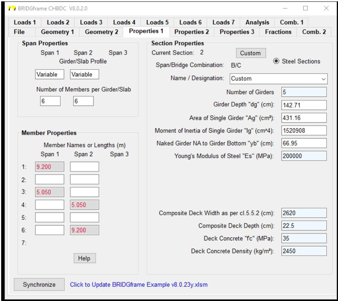
When more than one element has the same section properties, the elements can be grouped prior to synchronizing. First one element is selected and assigned properties. Hover your cursor over another element box and click your left mouse button to open the Modify Properties popup and select Current. Repeat until all elements are included in the group of same section properties. (see Appendix 7)
