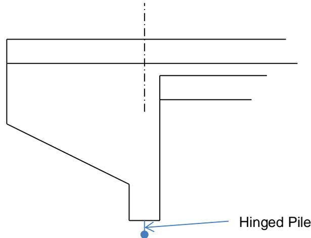
Integral Abutment with Hing between pile and abutment:
